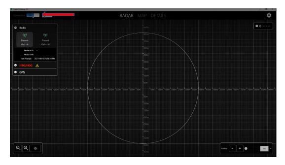
4. Any discrepancies / Fault will be seen as RED as shown in below picture (see RED arrow): In this picture we can see Firmware & License has been expired. So, both the firmware & license need to be updated. The firmware version is decided by the Software version installed. When software patch is released then we should make sure that gate way firmware is also updated. In this document we will see how the firmware is updated.
